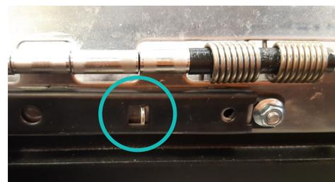
*The quick release latch enables easy removal of the SMARTtill Unit from the baseplate*
