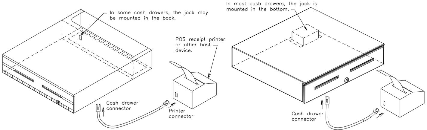
Interface cables are sold separately. Each cable is pinned, terminated, and labeled for the proper host device. Refer to the APG Connectivity Guide and the CD-\*\*\* Cable Pinout Guide for more information.
