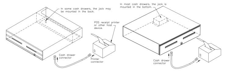
Interface cables are sold separately. Each cable is pinned, terminated, and labeled for the proper host device. Refer to the APG Connectivity Guide and the CD-\*\*\* Cable Pinout Guide for more information.
